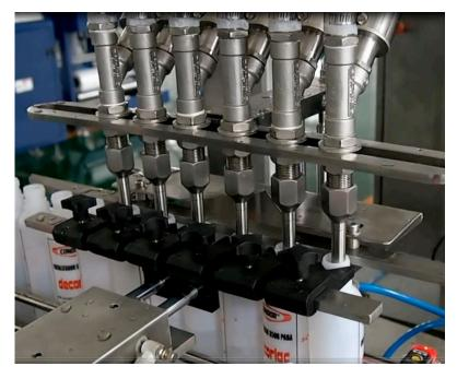
Subsequently, the product is pumped to the filler through an Atex pump, which will be "Class II" classified and will proceed to fill bottles from 50ml to 1 litre with a high precision volumetric filling system. After filling, bottles must be covered, using a versatile capper able to feed and thread the flip-top caps as well as thread the pumps cuppers which were fed manually.
